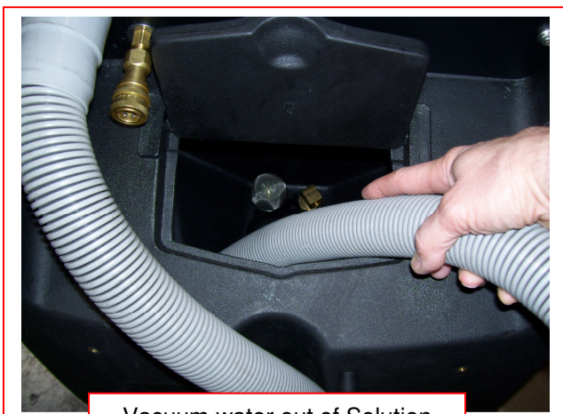
Vacuum water out of Solution Tank
