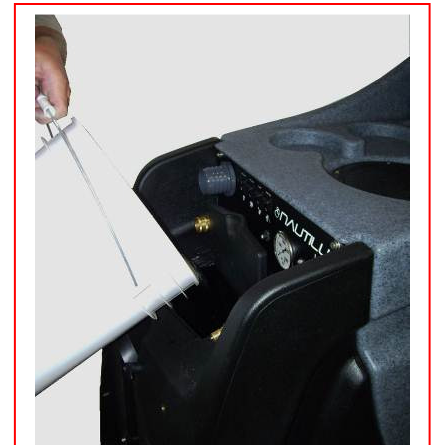
Pour 2 or 3 gallons of clean water into Solution Tank
